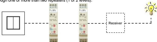
a) On the receiver, activate the slave RTL mode by a short press (approximately 0,5s) on **LRN** and **CLR** simultaneously. This mode is confirmed by the flashing (orange) regular of **LED**; then short press (approximately 0,5s) **CLR**. This mode is confirmed by the red **LED** flashing.
