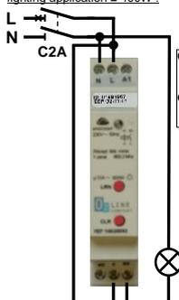
Connection drawing for a resistive load application ≤ 2300W :
